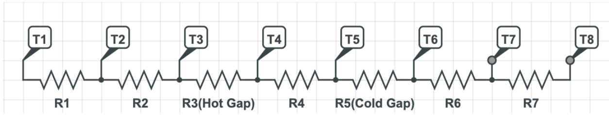
Figure 3: The circuit analogy employed into heat transfer.
